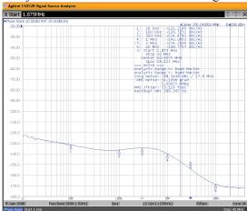
156.25MHz with 251fs<sub>RMS</sub> for phase jitter for 12kHz to 20MHz integration range
