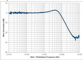
The jitter attenuation works like a low-pass filter for frequency modulated signals or noise. The bandwidth for this low pass filter is 500kHz with a 12dB/octave slope above 500kHz. At about 6MHz the noise floor of this measurement is reached but in reality, the attenuation continues with the 12dB/octave slope.
