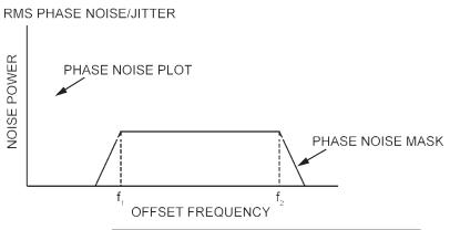
RMS JITTER = VAREA UNDER THE MASKED PHASE NOISE PLOT
