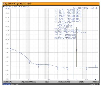
Output Clock from ABMJB-903: The 3MHz spur is attenuated by 20dB, resulting in a phase jitter reduction from 1.1ps to 0.10ps for 1.875MHz to 20MHz integration range
