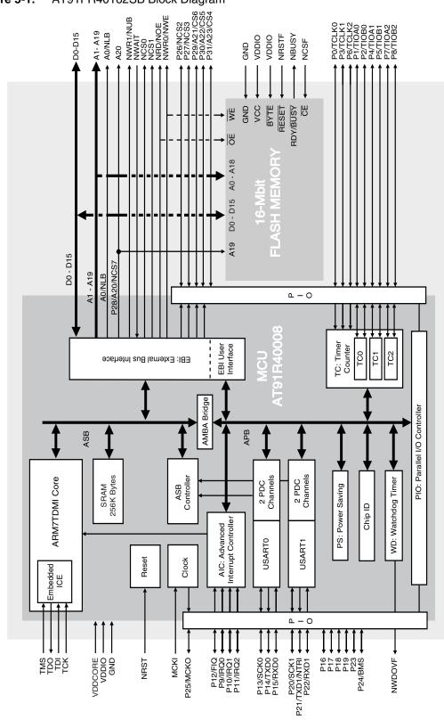
Figure 5-1. AT91FR40162SB Block Diagram
