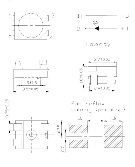
Note: Tolerances unless mentioned ±0.1mm. Unit = mm
